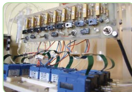
(b) The pumping system for the microfluidic platform, for pumping approx. 2 µl/min
