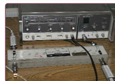
Measuring test set for S11 scattering parameter
