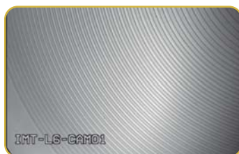
Fresnel lenses (operation in transmission) replicated in PDMS using a SiO 2 master
