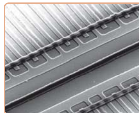
Detail of the MSM photodiode (interdigitated structure integrated with the SU-8 optical guide).
