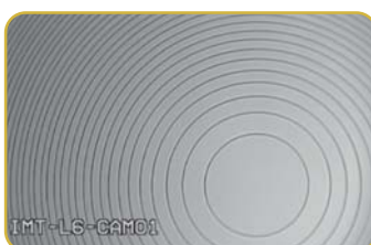
Fresnel lenses (operation in transmission) replicated in PDMS using a SiO 2 master
