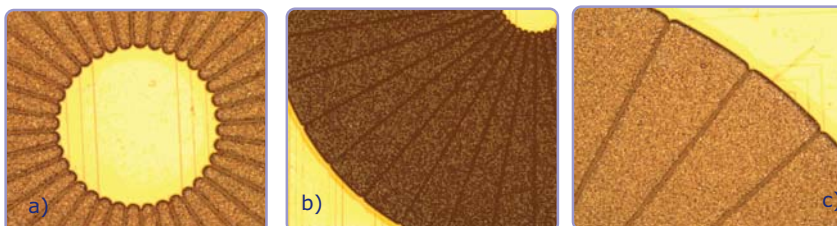
Silicon microprocessed micro-heat sink test structure (using electroplated Cu), (a) at the center, \varnothing_{in} = 0,6 \text{ mm} , (b) center-outside, (c) at the outside, \varnothing_{out} = 4 \text{ mm} .
