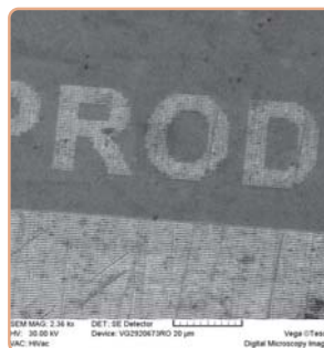
SEM micrographs of authentication stamps used in food industry.
