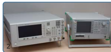
Upgraded to 110GHz set-up for "on wafer" S parameters measurements (left), Generator up to 110 GHz and the Spectrum Analyzer up to 110 GHz (top).
