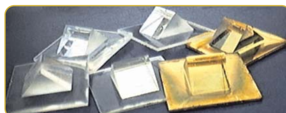
Prisms for SPR sensors obtained in epoxy rewsin using a glass original (master) and a PDMS mold (negative copy).
