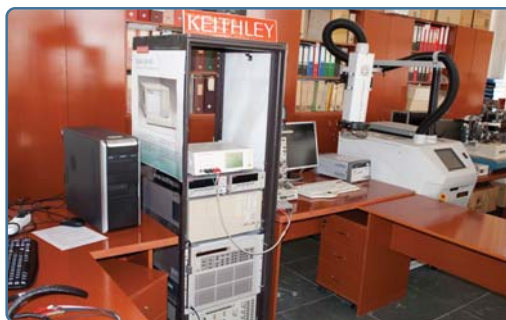
The experimental set-up for electrical characterization at various temperatures: Equipment for electrical measurement 420 SCS (left) and Equipment for temperature conditioning ThermoStream (right).
