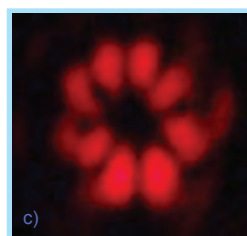
a) White light interferometry image of a diffractive optic element generating an optical vortex with m=4 . Optical vortex with m=4 . c) Interference of two vortices with m=4 si m=-4 .
