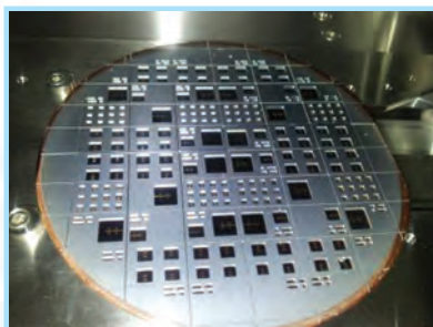
Back side view for the test structures fabricated in 2013 through silicon micromachining
