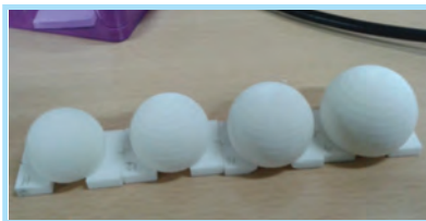
Photo of polyamide lenses fabricated through 3D printing (cooperation with L5- Dr. G. Moagar)
