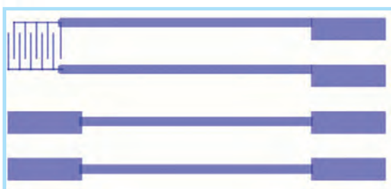
Layout for the structure of impedimetric sensor and pH sensor the distance between electrodes is 50 \mu\text{m}
