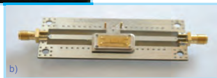
Surface Acoustic Wave biosensor: a) Side view of the biosensor; b) Calibration device; c) Transmission parameters; d) Reflection coefficients
