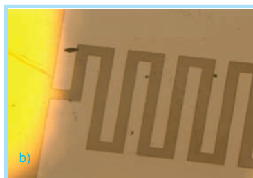
a) Absorption of metamaterial structures in infrared region. b) Bolometer sensor based on patterned YBCO thin layers c) Variation of polarization current intensity with the level of the infrared irradiation.
