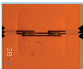
(a) analytical modeling for 1, 2 and 3 cells; (b) fabricated membrane supported filter structure; (c) experimental results for a 2-cell filter
