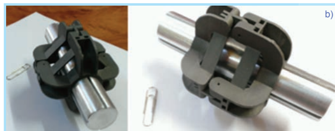
b.) The torque sensor mounted on the metallic shaft.
