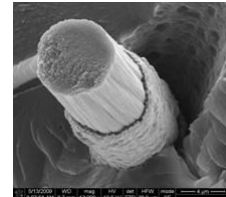
L V SEM micrograph of Ni coated carbon fibers embedded in resin
