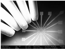
Pt lines deposition by EBID- 50nm line width
