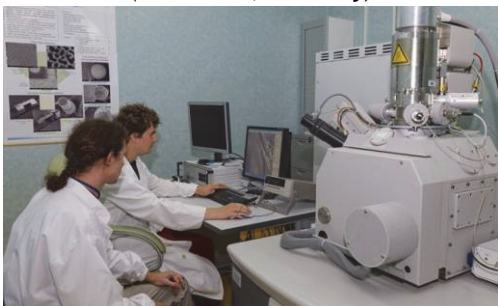
Field Emission Gun Scanning Electron Microscope (FEG-SEM) - Nova NanoSEM 630 (FEI Company, USA)
