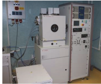
Electron Beam Evaporation and DC sputtering system - AUTO 500 (BOC Edwards, UK)
