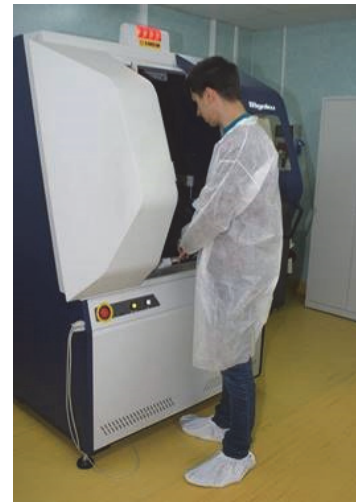
X-ray Diffraction System (triple axis rotating anode) - SmartLab - 9kW rotating anode, in-plane arm (Rigaku Corporation, Japan)
