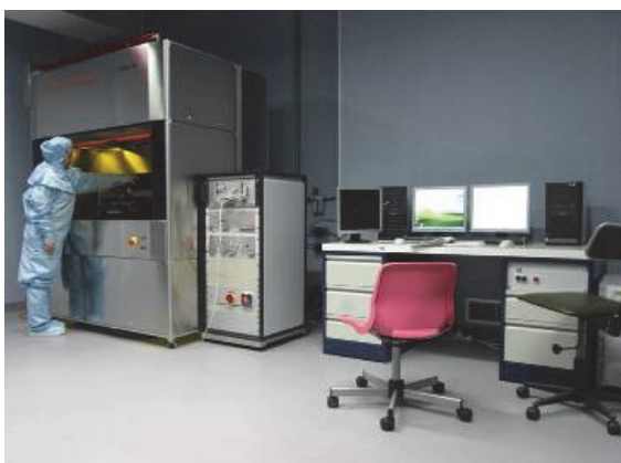
Laser lithography system - DWL 66 fs, direct writing laser, high resolution pattern generator (Heidelberg Instruments Mikrotechnik, Germany)
