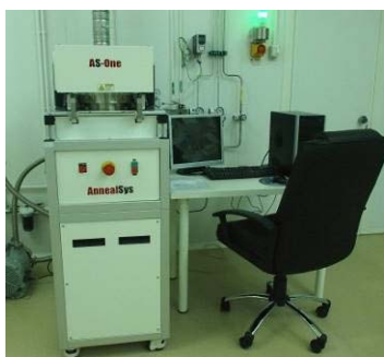
Low Pressure Chemical Vapour Deposition Equipment (LPCVD) - LC100 (AnnealSys, France)
