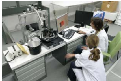
Scanning Probe Microscope - NTEGRA Aura (NT-MDT Co., Russia)
