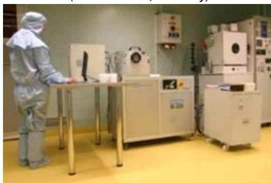
RIE Plasma Etcher - Etchlab 200 (SENTECH Instruments, Germany)
