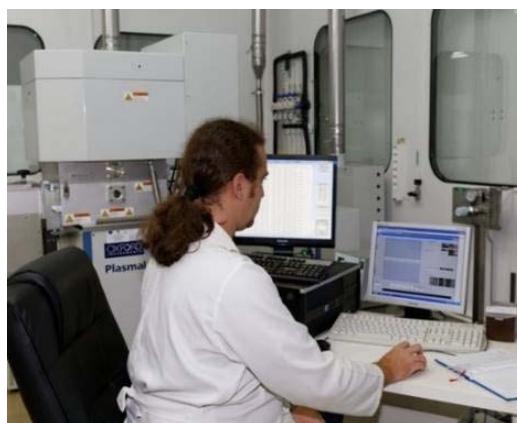
DRIE - PlasmaLab System 100 (Oxford Instruments, UK)
