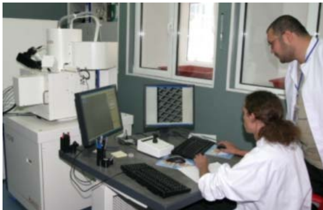
Electron Beam Lithography and nanoengineering workstation - e_Line (Raith, Germany )
