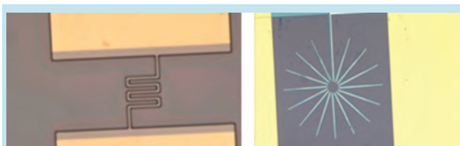
The optical microscope image of the meander source The optical microscope image of the thermopile in a "star" configuration.
