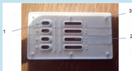
Fig 7. Capsule cover: 1. Slot area sample, 2-point measuring area, 3 guide pin
