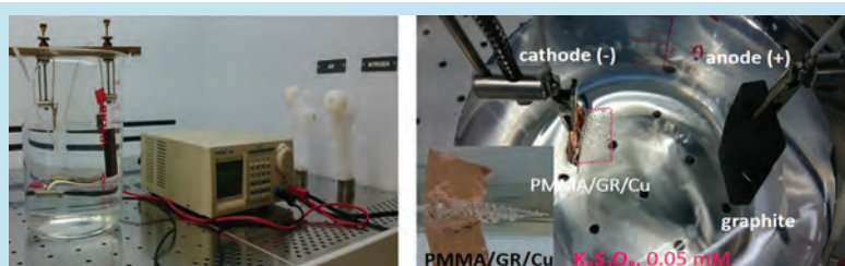
Electrochemical delamination home-made system of graphene transferred from Cu foil: overview (left) and enlarged view (right), in inset, image showing the peeling of the “whole film” PMMA/graphene from the Cu foil. (Contact Dr. Anca Istrate, Dr. Monica Veca, Dr. Florin Nastase)
