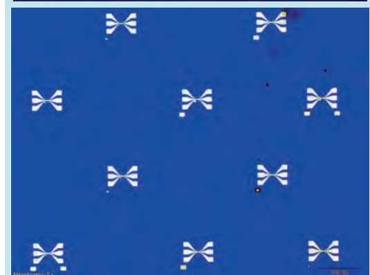
Balistic diodes on graphene (graphene on Si/SiO 2 - 300 nm SiO 2 thickness)
