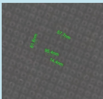
Core-shell nanodot arrays: a) Si/SiO 2 /(Au)/TiO 2 , b) Si/SiO 2 /Au/TiO 2 /ZnO
