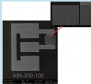
SEM photos of a SAW structure with coplanar waveguide type pads manufactured on GaN/Si wafers having IDTs with finger/interdigit spacing width of 200 nm and 100 \mu\text{m} finger length
