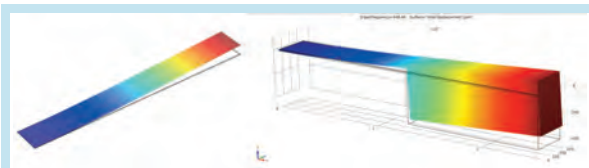
Fig 10. Simulations on the resonating beam for power generation: simple (left) and inertial (right)
