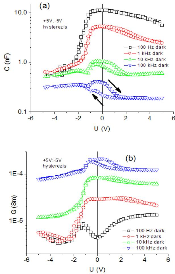
**Fig. 4.** Dark C–V and G–V characteristics for a sample with macrocrystalline PbS.
