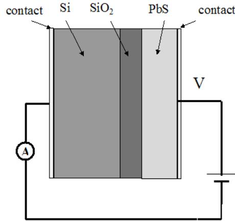
**Fig. 2.** Heterostructure Si/SiO<sub>2</sub>/PbS under transversal bias conditions.
