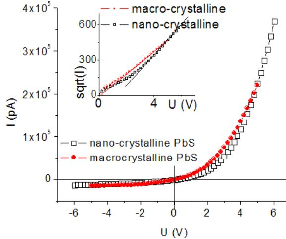
**Fig. 3.** Transversal I–V curves for the heterostructures in Fig. 2.
