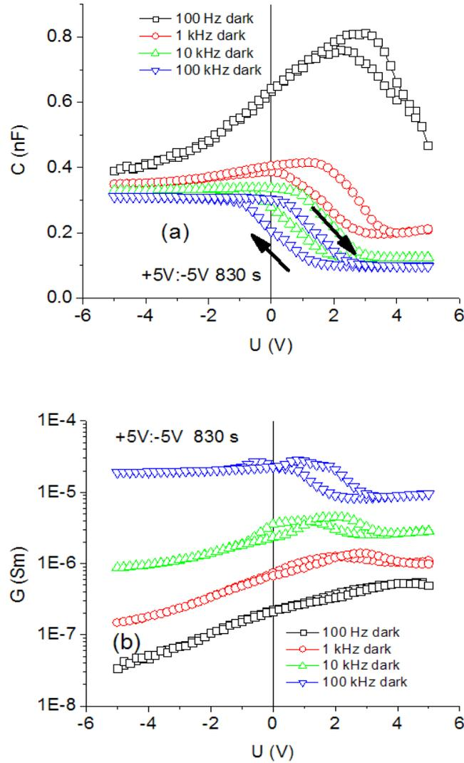
**Fig. 5.** Dark C–V and G–V characteristics for a sample with nanocrystalline PbS.
