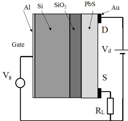
Fig. 7. Biasing scheme for field-effect measurements.
