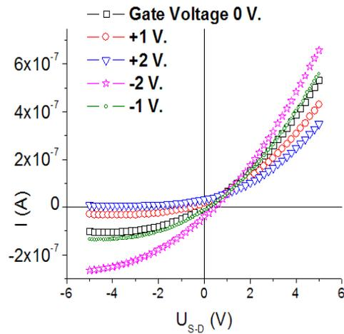
Fig. 8. Dark I-V characteristics S-D having the gate voltage as a parameter.
