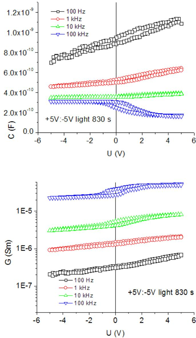
**Fig. 6.** C–V and G–V characteristics for a sample with nanocrystalline PbS with sample illumination.
