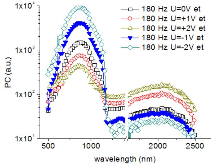
**Fig. 9.** Photocurrent spectrum for sample B with the gate voltage as a parameter.
