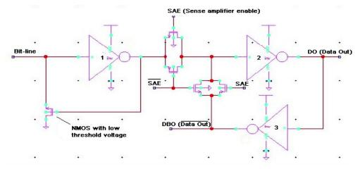
Fig. 5. Possible circuit schematic of sense amplifier.
