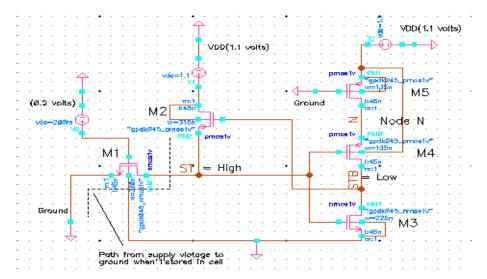
Fig. 9. Path from supply voltage to ground.
