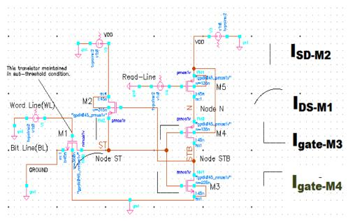
Fig. 3. Leakage current in idle mode when '0' stored in cell.
