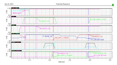
Fig. 6. Waveform of new cell during read cycle.
