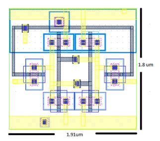
Fig. 7. Layout of 6T cell using 45 nm technology.
