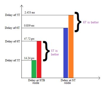
Fig. 11. Delay Comparison between 5T and 6T.
