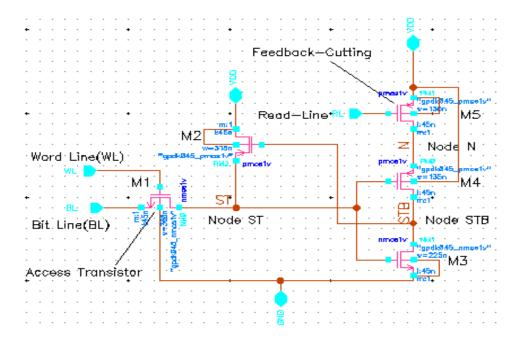
Fig. 2. New 5T SRAM cell in 45-nm technology node.
