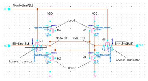
Fig. 1. SRAM cell current in 6T SRAM cell.
