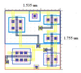
Fig. 8. Layout of 5T cell using 45 nm technology.
