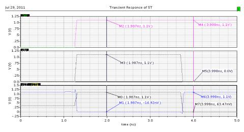
Fig. 4. Waveform of new cell during write cycle.
