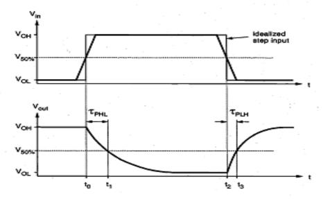
Fig. 10. Input and output voltage waveforms of a typical inverter, and the definitions of propagation delay times. The input voltage waveform is idealized as a step pulse for simplicity.
