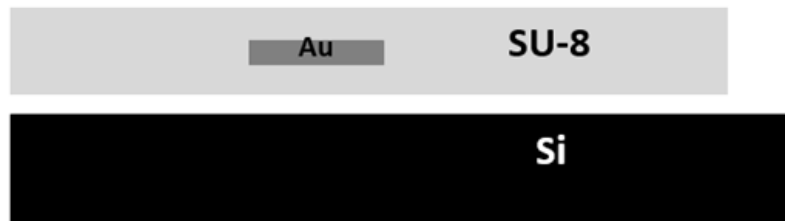
Fig. 8: Schematic cross section of the arms of the microgrippers after fabrication [ [6], [23].
