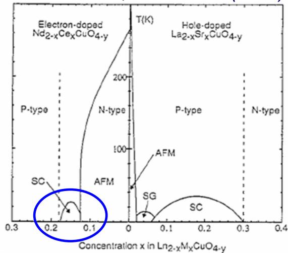
$I_c$  vs. dopant concentration phase diagram for  $T'-Ln_{2-x}Me_xCuO_4$
