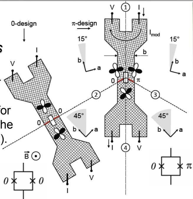
For  $d_{x^2-y^2}$ -wave symmetry: the  $\pi$ -SQUID consists of one 0-Josephson junction and one  $\pi$  Josephson junction ( $\pi$ -phase shift inside the SQUID loop).
