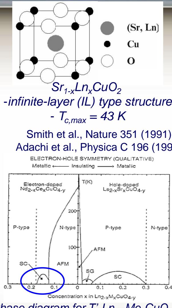
Phase diagram for  $T'\text{-}\text{Ln}_{2-x}\text{M}_x\text{CuO}_4$
