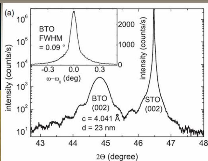
XRD  $2\theta/\omega$  and rocking curve scans of BTO/STO symmetric (002) reflection; film thickness estimated from Laue fringes
