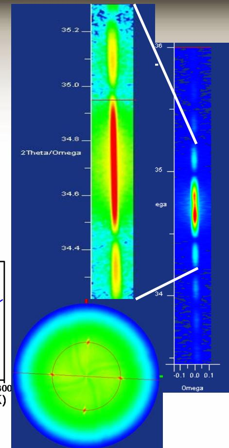
HRXRD rsm and pole figure of asymmetric (101) plane
