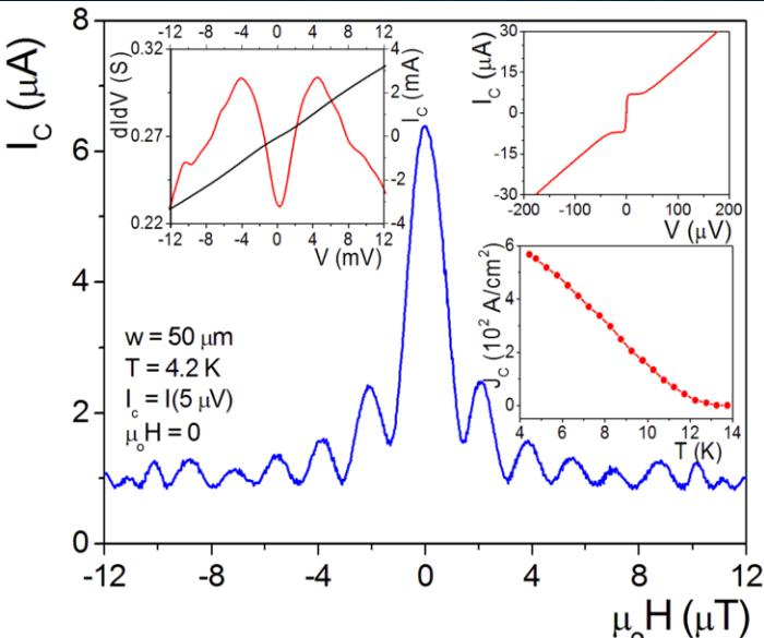
Symmetric 30°, [001] tilt grain boundary SLCO junction data
