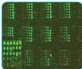
Silicon slides functionalized with poly-L-lysine: a) after spotting and b) washed after 60 minutes
