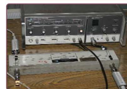
Measuring test set for S11 scattering parameter
