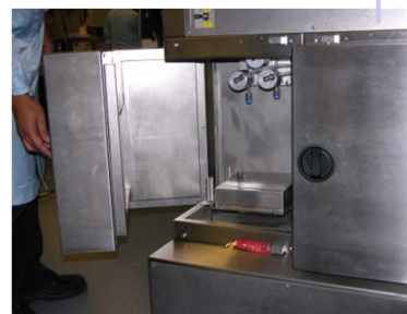
OpAL thermal system with two precursor delivery modules
